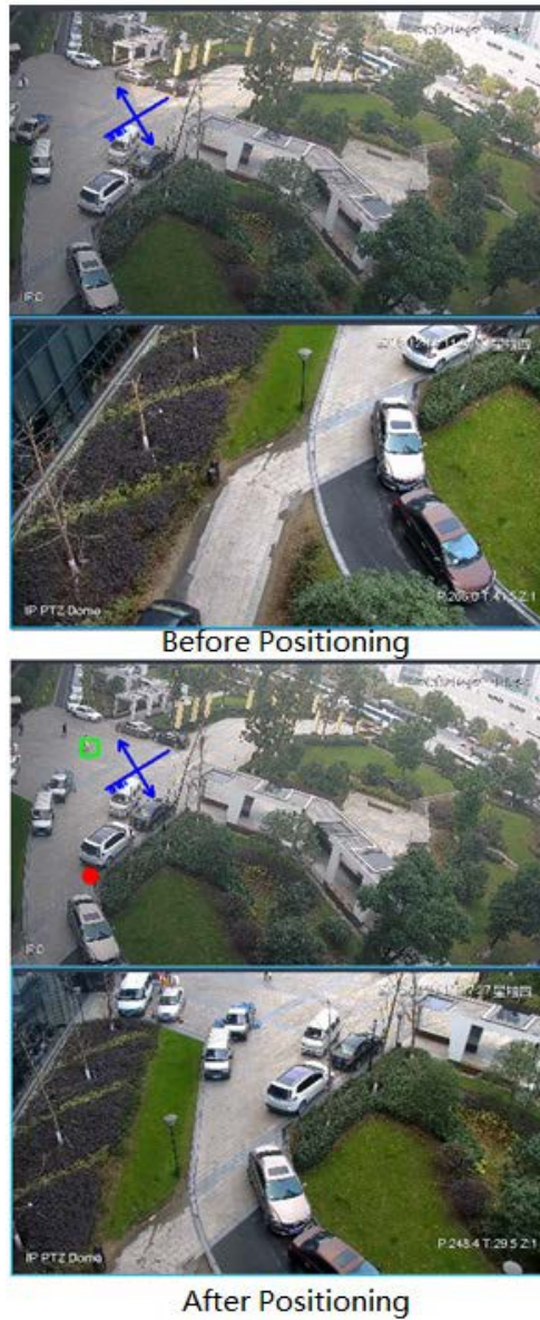
Figure 4-111 3D positioning (Zoom in after positioning)
